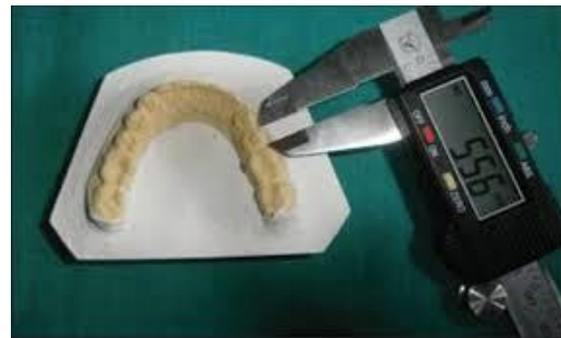
Figure 1: electronic digital veneer caliper used for the measurement of the MD width of teeth
